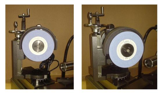
Attention: to change the working angle, the wheel must be in the top position.
