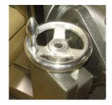
the wheel height can be adjusted to work inside the flutes
