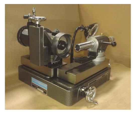
With the setting showed, **(Wheel removed to show the machine parts)** the machine acts as a regular two axes Cuttermaster.
